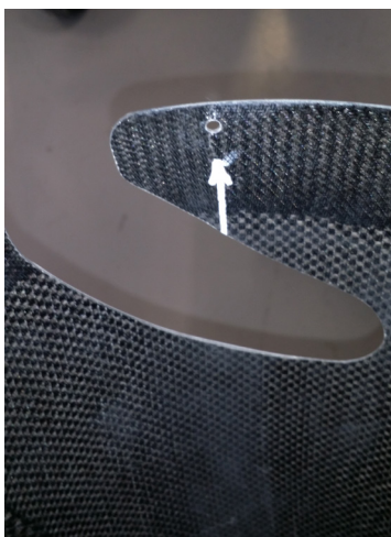
Figure 61-006 Marking on the inner side of the spinner
