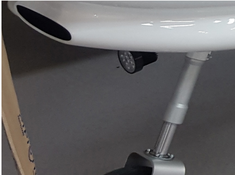
Figure 33-002 Example of landing light installation
