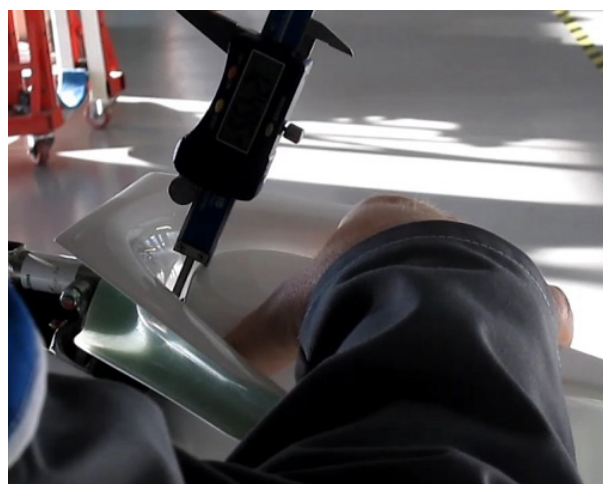
Figure 27-005 Rudder axial free play check
