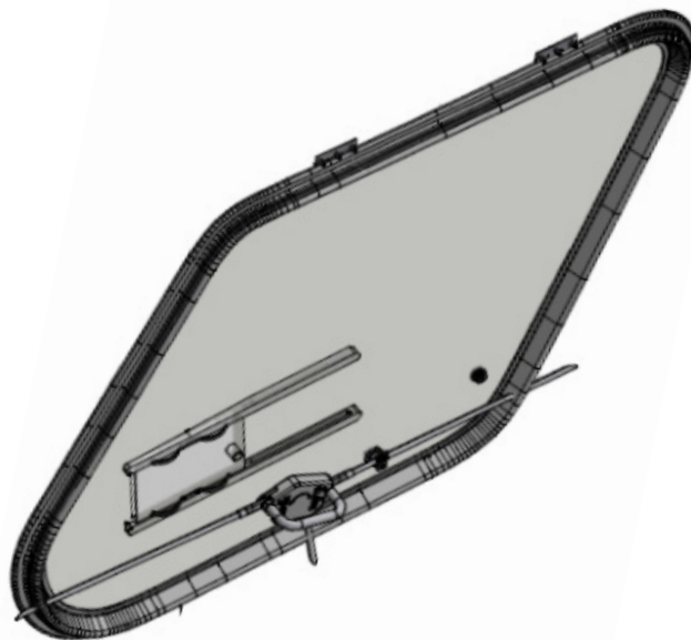
Figure 52-001b Door with new locking mechanism installed
