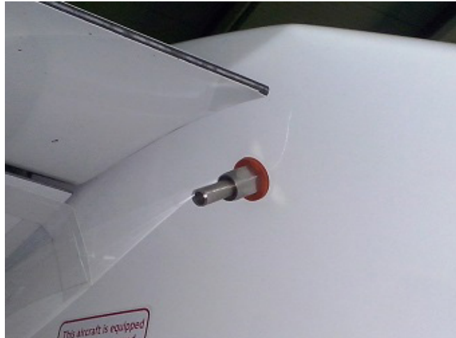
Figure 34-002 OAT sensor installation
