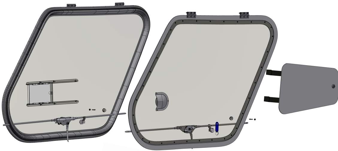
Figure 52-001a Doors with old locking mechanism installed
