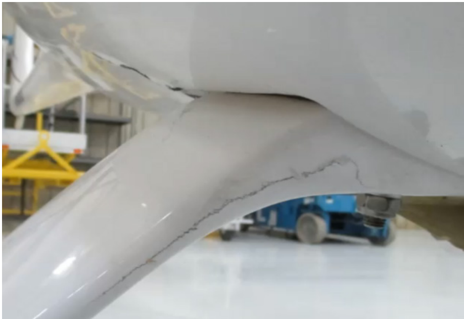
Figure 32-002 Example of a damaged main landing gear strut
