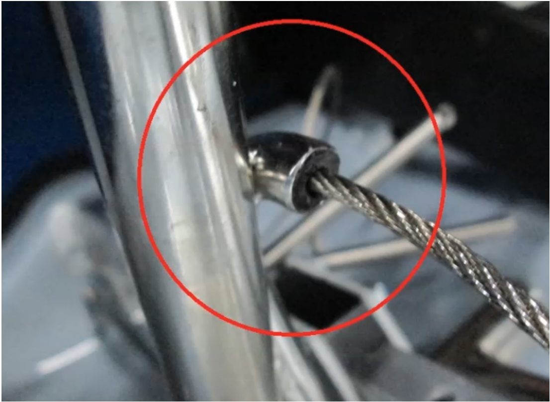
Figure 27-002 Upper pedal-rudder cable joint
