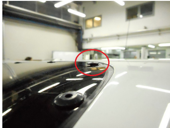
Figure 56-004 Example of loosened window rivet
