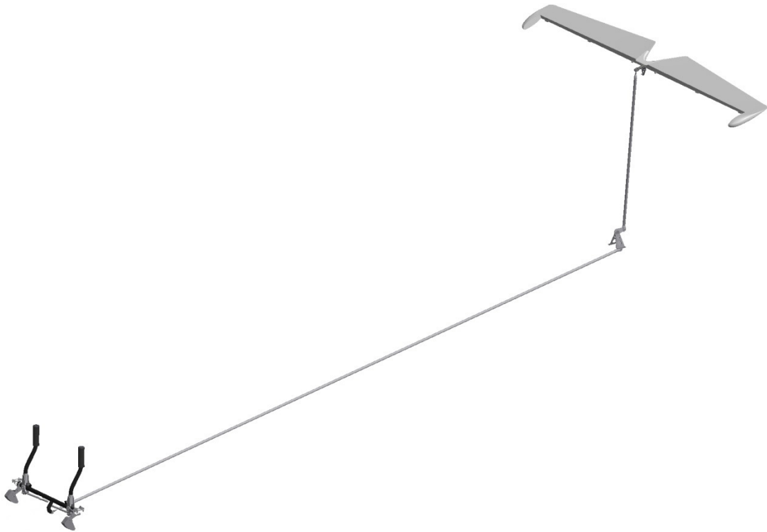
Figure 27-006 Elevator control system
