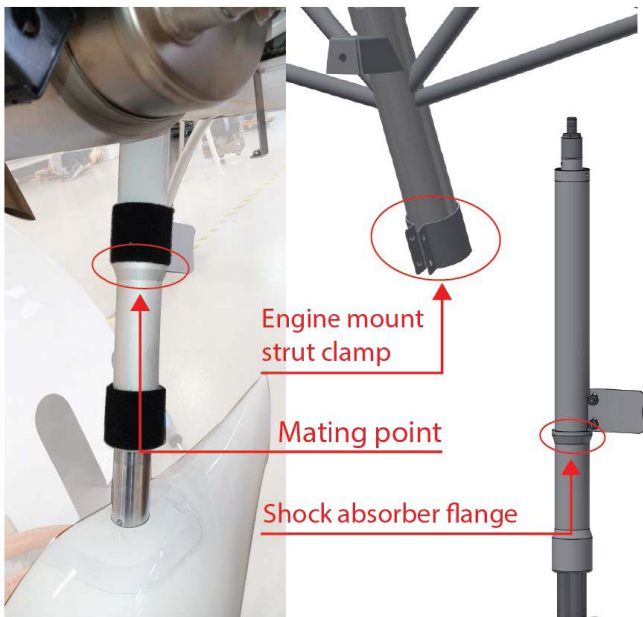
Figure 32-008 Inspection main focus points
