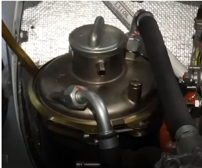
Figure 79-002 Example of oil tank installation orientation
