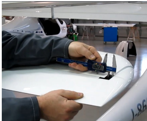
Figure 27-008 Elevator axial free play check
