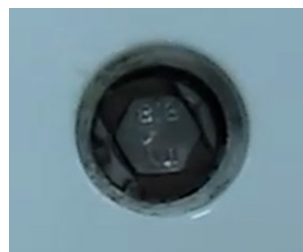
Figure 55-002 Attachment bolt assembly head orientation
