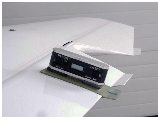
Figure 27-0016 Elevator deflection angle adjustment
