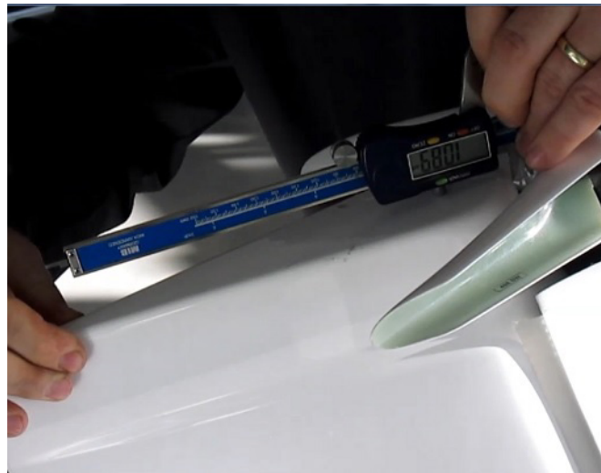
Figure 27-004 Rudder radial free play check
