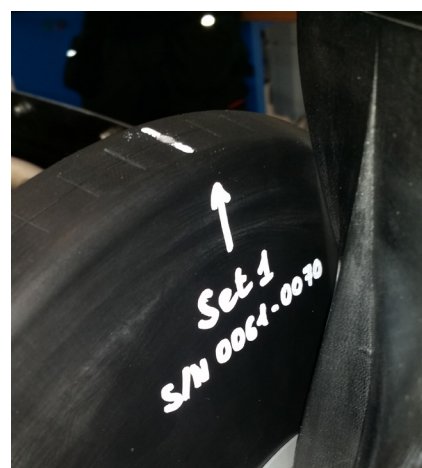
Figure 61-007 Marking on the spinner plate
