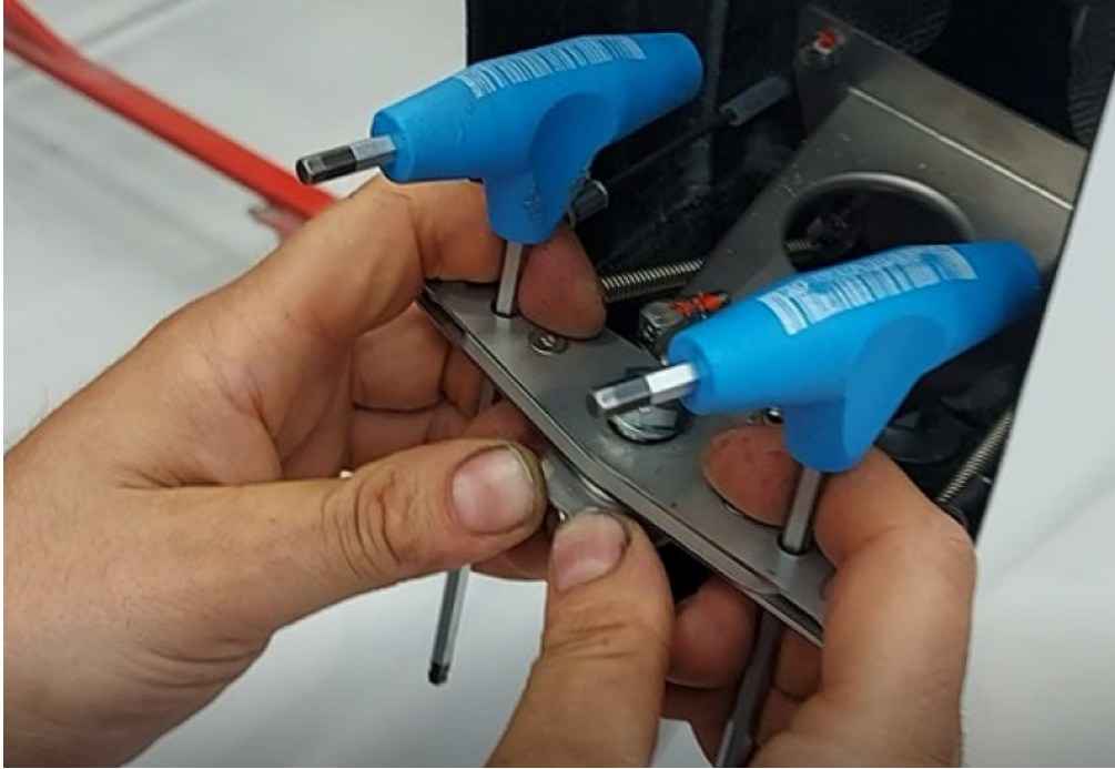
Figure 32-015 Rudder bellcrank installation
