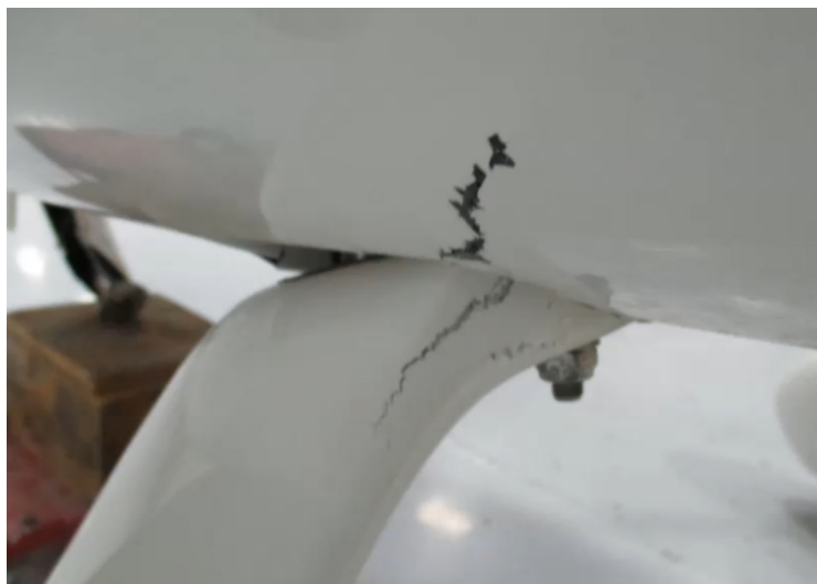
Figure 53-002 Example of fuselage main frame damage
