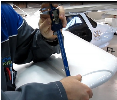
Figure 27-009 Elevator radial free play check
