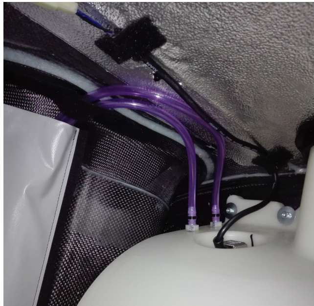
Figure 28-001 Fuselage fuel tank return and breather lines
