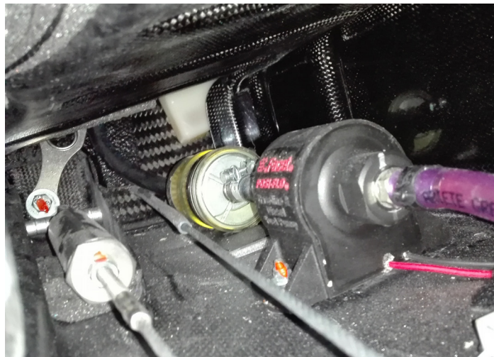
Figure 28-005 Fuel pump and filter below baggage compartment
