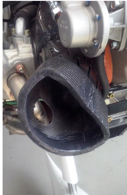
Figure 71-003 Example of ram cooling air intake
