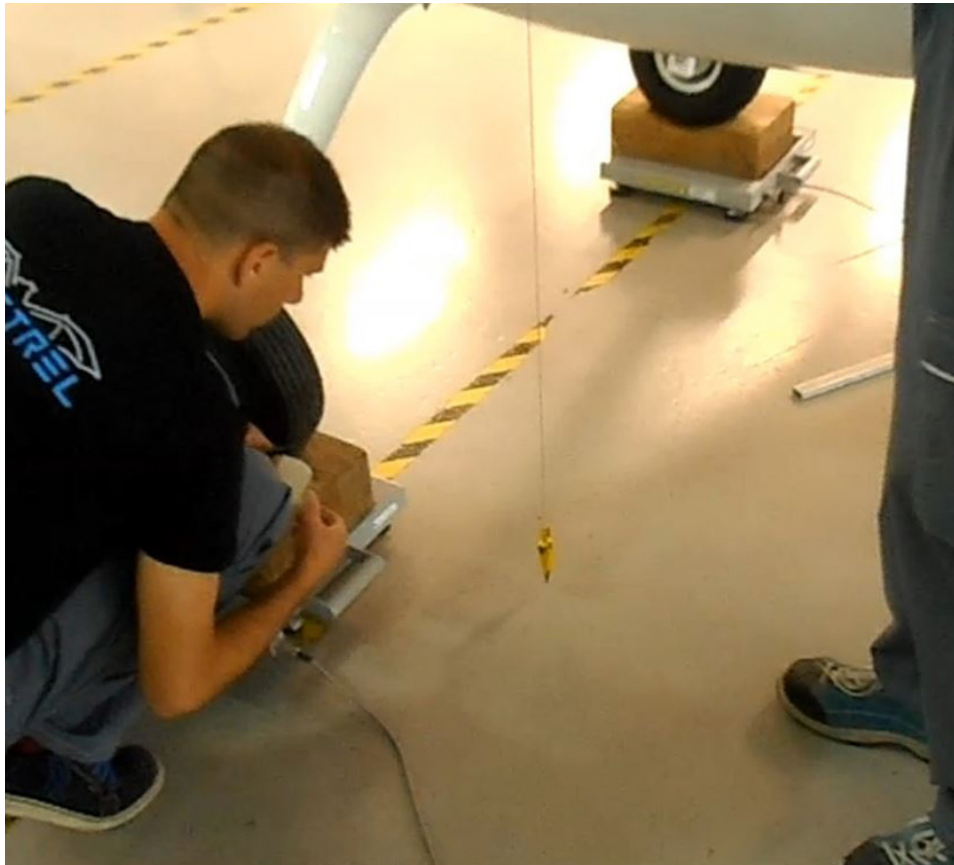
Figure 08-002 Plump bob from wing leading edge
