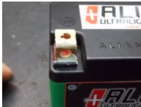
Figure 24-002 Example of battery terminal oxidation
