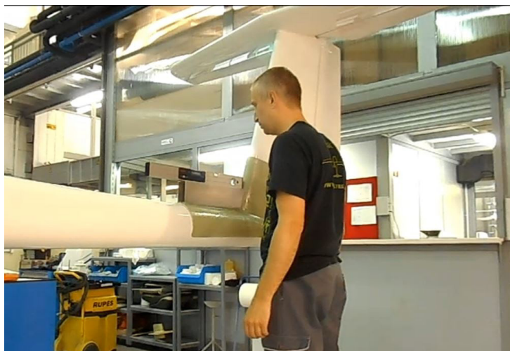
Figure 08-001 Leveling tool and spirit level setup
