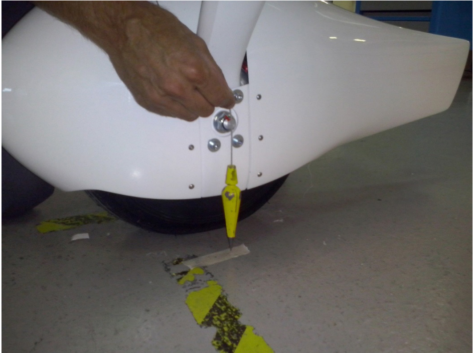
Figure 08-003 Plum bob from center of the MLG wheels - Illustrative only -
