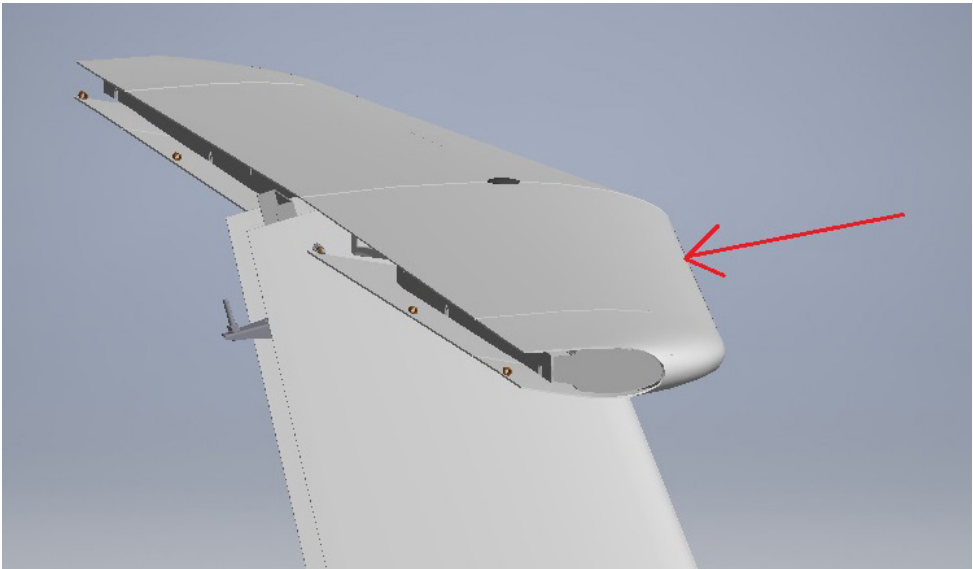
Figure 51-004 Horizontal stabilizer leading edge bonding line - illustrative purposes only -
