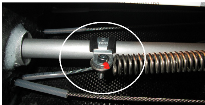
Figure 27-012 Elevator trim assembly spring fastening material
